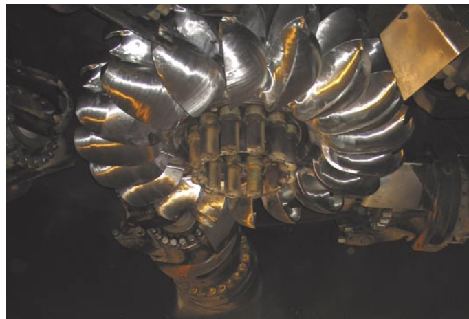
One of the Pelton turbine runners at EGEMSA's hydro power plant in Machu Picchu.
