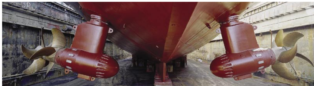
Rolls Royce azimuth thrusters mounted on a Scandlines ferry
