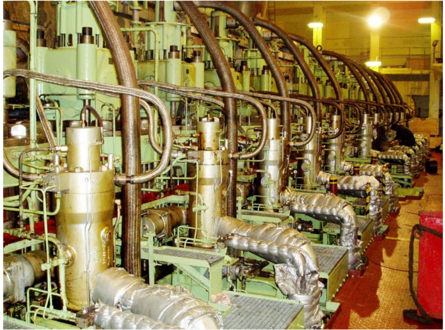
Top of the main engine of one of A.P. Moller - Maersk's container vessels.
