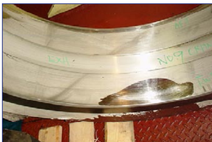
Crosshead - (1), crankpin - (2) and main bearings (3) are very sensitive to wear, which can ultimately lead to crucial damage to the crank shaft bearing (Example below).
