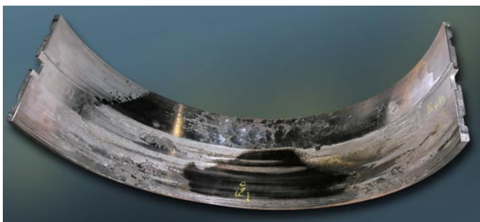
Bearing totally damaged due to steel-to-steel contact. Such a damage, with repair time up to 6 months, as well as damage and costs statistics from a large ship insurer clearly demonstrated the need for condition monitoring.
