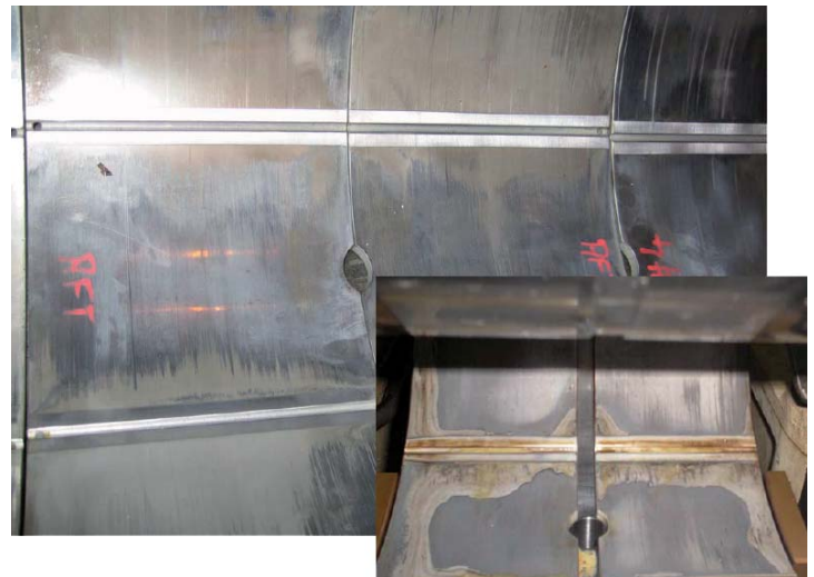
Bearings damaged as a result of water contamination of the system oil. Courtesy: MAN Diesel.
